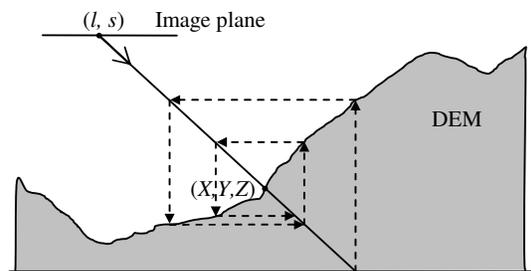
Figure 1. 3D point positioning from single image and DEM
