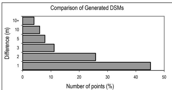
Figure 5. Comparison of ISAE and MPGC DSMs.
