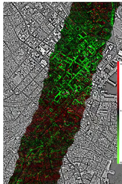
Figure 4. Difference map between the ISAE and MPGC generated DSMs.
