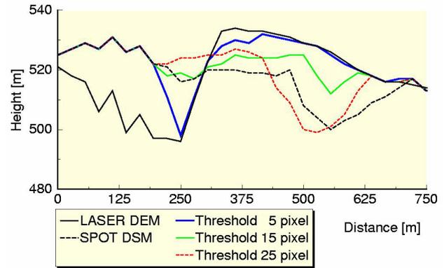
Figure 5. Cut through the northern part of area ‘Taching’ in the reference laser DEM, the SPOT DSM, as well as three integrated DSM with different thresholds as given in the legend.
