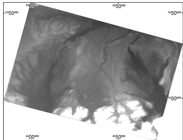
Figure 1. DSM resulting from matching of a SPOT stereo image pair acquired on October 1, 2002 and following triangulation of 7.7 Mio. object space points.
