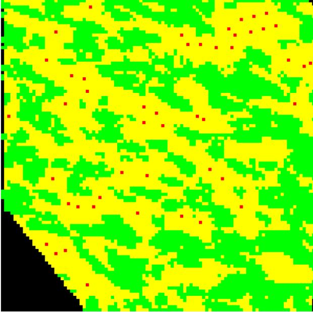
Figure 3. Resulting distribution by iterative point integration. Green = Pixel with SPOT 3D point. Red = Pixel with integrated point ( $n_i = 48$ ). Yellow = Pixel to interpolate. Threshold = 20 pixels.
