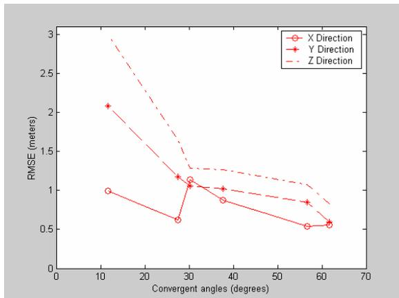
Figure 4. The relationships between ge positioning accuracies and convergent angles.
