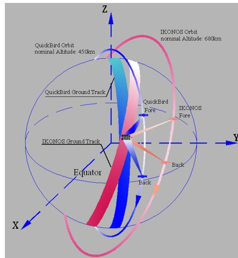
Figure 1. Orbital Geometry of QuickBird and IKONOS Satellites (inclination angles: QuickBird is 97.2°; IKONOS 98.1°; the difference is exaggerated in illustration)
