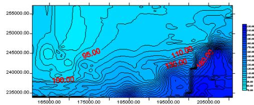
figure 4 . Illustration of the piezometric surface.
