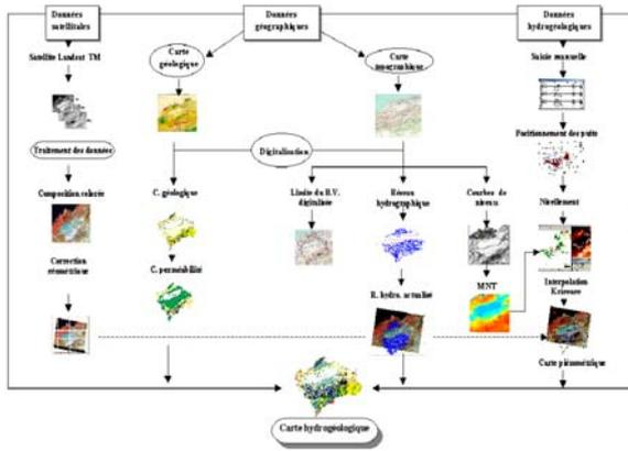
Figure 2 . Flow chart adopted for the development of the hydrogeologic map
