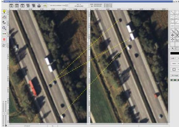
Figure 2. XDibias visualizer to measure vehicles in subsequent images
