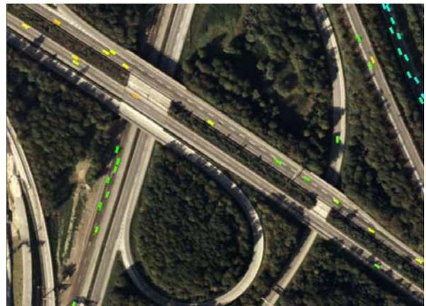
Figure 5. Clipping from a film animation showing moving vehicles on a freeway interchange north of Munich, blue=slow vehicles, orange=fast vehicles
