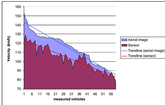
Figure 4. Velocity comparison for single vehicles measured with radar sensors and aerial images (linear regression for 60 cars at two signboard bridges)
