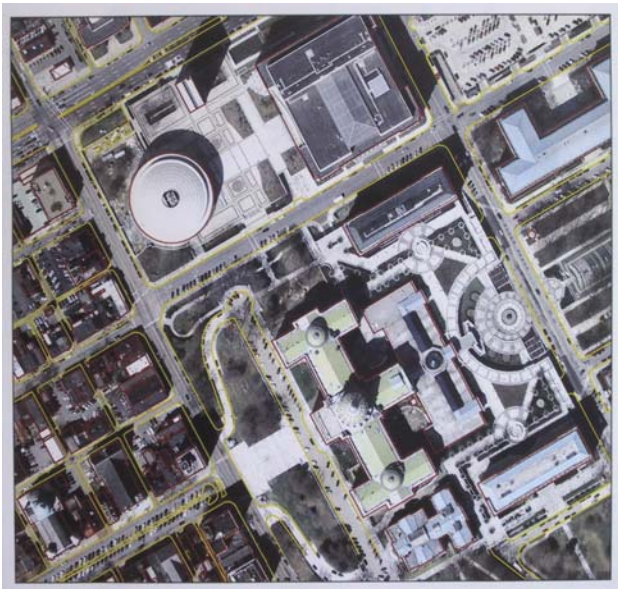
Fig. 9: True Ortho Map based on 30 cm GSD DSM
