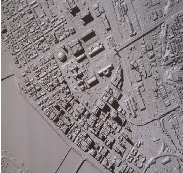
Fig. 8; DSM derived from 30 cm GSD ADS40 3-line image
