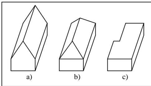
Figure 8. Building roof styles: a) gable, b) hip and c) flat
