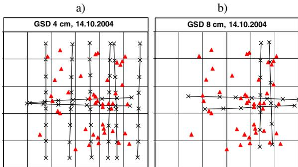
Figure 2. Block structures and GCP configurations at Sjöckulla large-scale test-field; 44 GCPs. a) Geotec, GSD 4 cm; comprehensive block and b) Geotec, GSD 8 cm; cross-block (other two blocks with 8 cm GSD had similar structure).
