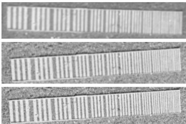
Figure 7. Example of resolution bar targets from simultaneous UltraCamD and RC20 images; GSD 4 cm flight (14.10). From top to bottom: UltraCamD, RC20 with 20 µm pixel size and RC20 with 10 µm pixel size.
