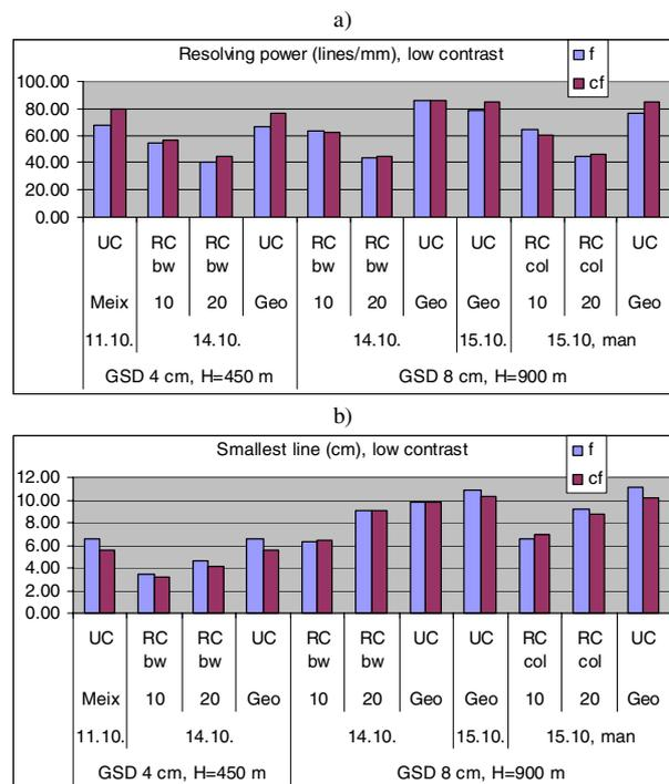
Figure 5. Spatial resolution of 4 cm and 8 cm GSD flights in flying direction (f) and cross-flight direction (cf). a) Average resolving power in lines/mm. b) Average smallest resolvable line in cm. (bw: black/white film, col: color film, man: manual mount, 10: 10 µm pixel size, 20: 20 µm pixel size).
