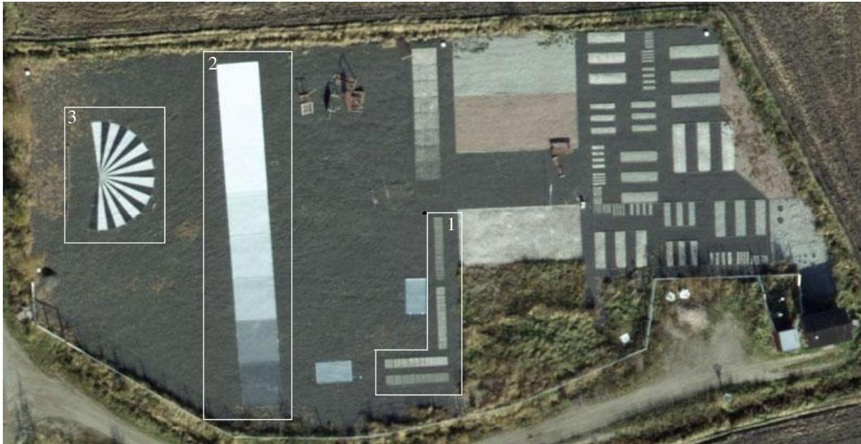
Figure 1. Overview of Sjöckulla test site during testflights. The test figures used in this study are: 1) permanent dense spatial resolution test bar targets, 2) transportable grey scale with 8 steps and 3) transportable Siemens star. Photo by Meixner.
