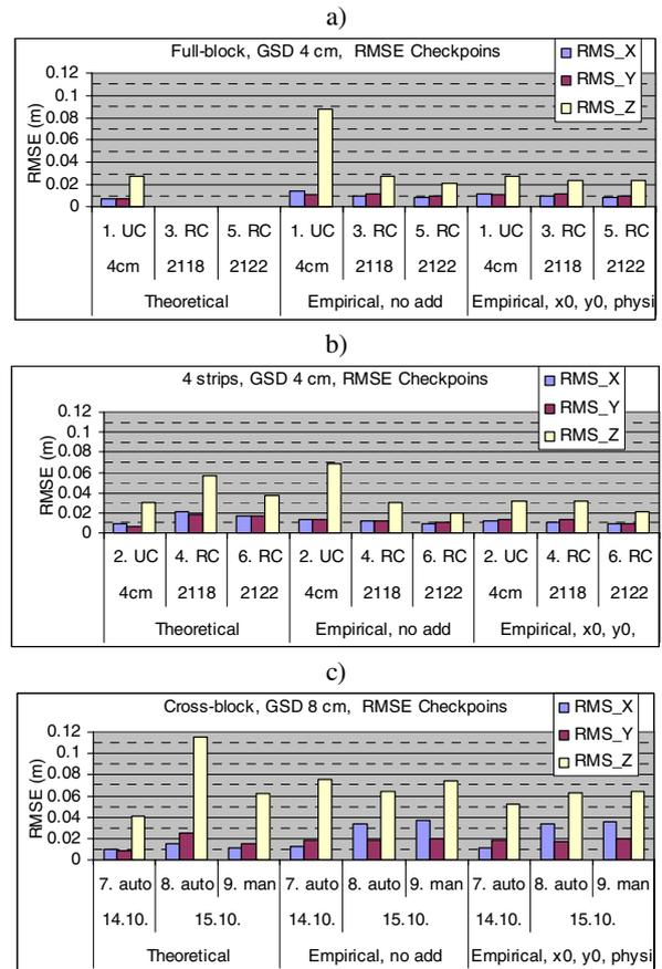
Figure 4. Point determination accuracy. Theoretical accuracy of point unknowns and empirical accuracy are shown. a) Comprehensive blocks (1, 3, 5), b) block with 4 strips (2, 4, 6). c) Cross-shaped blocks with 8 cm GSD (7, 8, 9).
