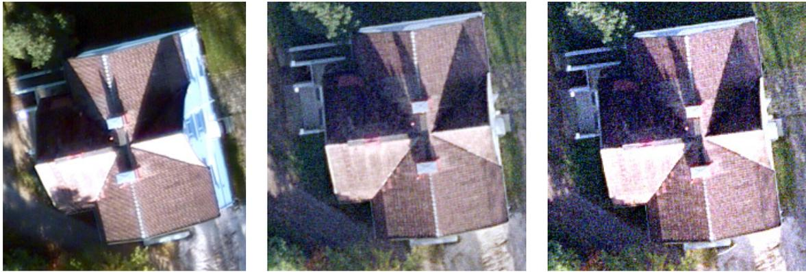
Figure 6. Detail from GSD 8 cm flight (15.10). Left to right: UltraCamD; RC20 with 20 µm pixel size; RC20 with 10 µm pixel size.
