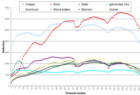
Figure 4: Spectra of roof surfaces (directly taken from the real HyMap data set)
