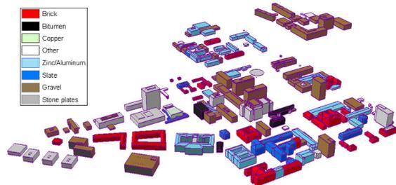
Figure 1: The main campus of Karlsruhe University (approx. 1km x 0.5 km) CAD model generated from aerial photogrammetry
