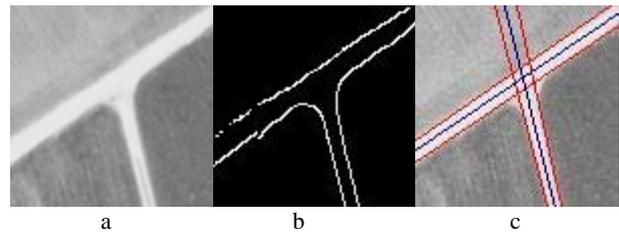
Figure 6: Three-arm junction: a) original image, b) edges, c) detected straight lines (red) and the computed centerline (blue)
