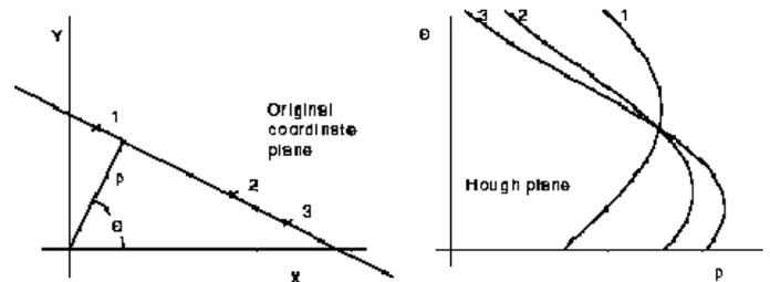
Figure 1: The coordinate system of the original image and the Hough-space [1]
