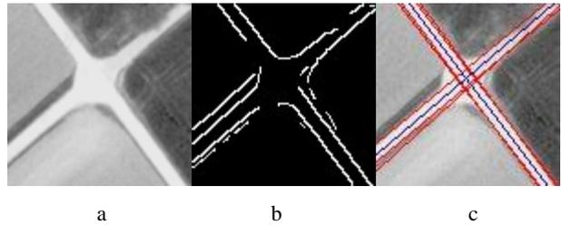
Figure 5: Four-arm junction: a) original image, b) edges, c) detected straight lines (red) and the computed centerline (blue)
