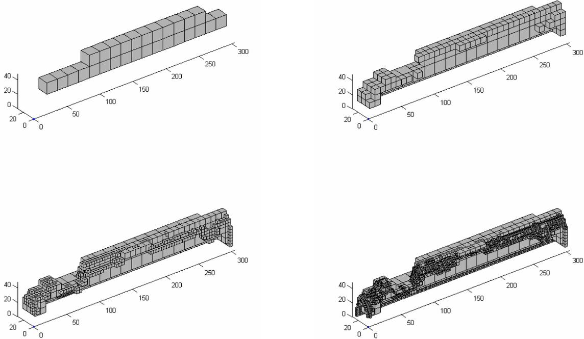
Figure 4. Iterative refinement in truck visualization (modelling) using the voxel pyramid structure
