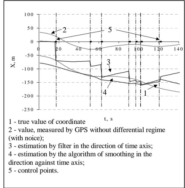
Figure 2. Example of the estimation of coordinate X.
