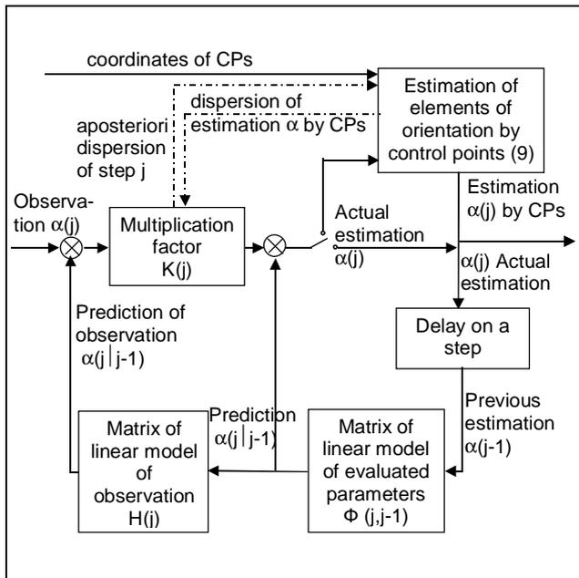
Figure 1. Block diagram of discrete nonstationary filter for estimating the elements of exterior orientation.
