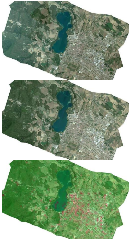
Figure 2. Banyoles image block Baix/Mig with 42 images corrected by the Pepita software of IGN/ENSG. Top: image mosaic without radiometric correction. Center: Pepita radiometric aerial triangulation with radial component. Bottom: residual values at tie points; highest values are in red and lowest in green. (Chandelier, 2010)
