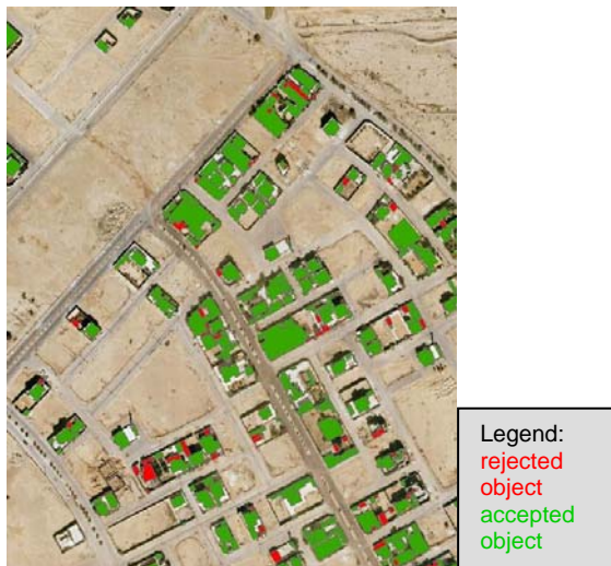
Figure 7: Orthophoto superimposed with traffic light diagnostics (cp. Figure 3).
