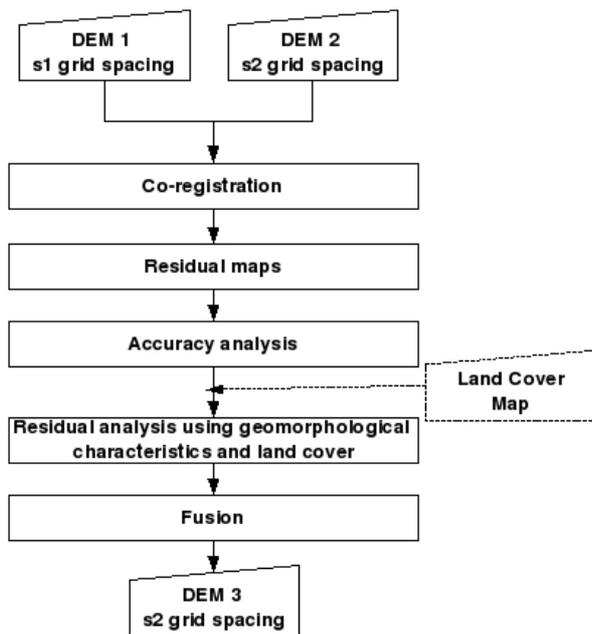
Figure 1: Workflow of the DEM fusion approach.
