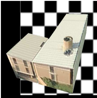
Figure 5. 3D building models textured using Pictometry oblique images block
