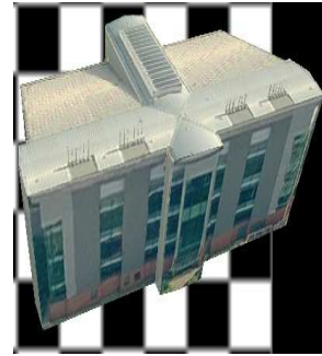
Figure 7. 3D building models textured using Pictometry combined block, very good texturing quality of roofs and facades
