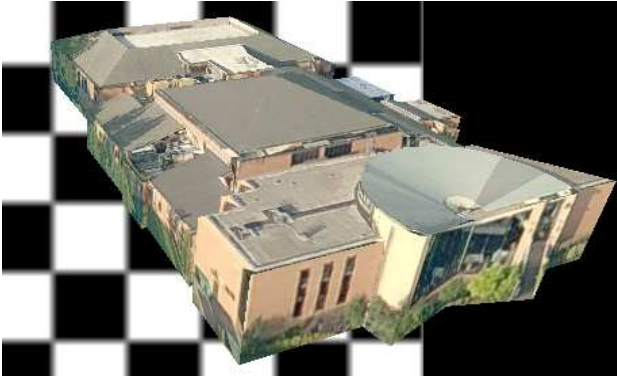
Figure 10. Texturing quality is affected by vegetation close to the building facades
