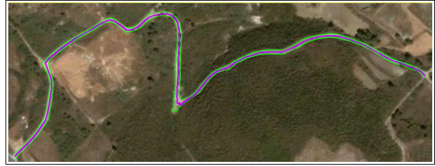
Figure 4. Optical: road edges (lines in green), road centerline (in magenta).
