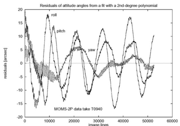
Figure 1: Oscillations on pixel scale of MOMS attitude angles measured by gyros (MOMS pixel: 8 arcseconds IFOV)
