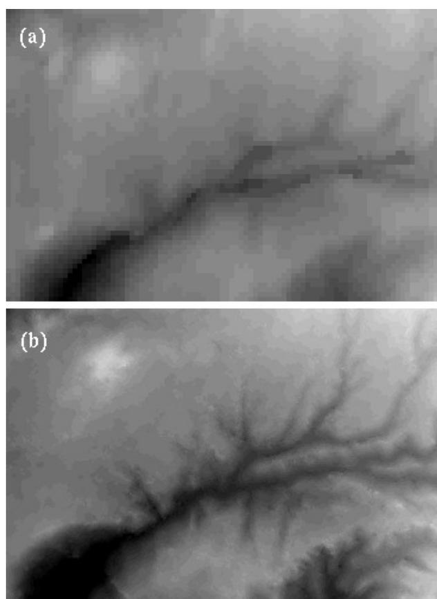
**Figure 3: Comparison of DEM subarea (9 km x 6 km) of Afghanistan strip: input DEM used for GCP height extraction (a) versus MOMS DEM (b)**
