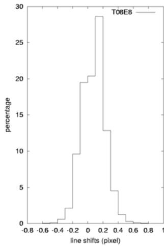
**Figure 4: Histogram of line shifts between channels 6/7 for MOMS data take T08E8**
