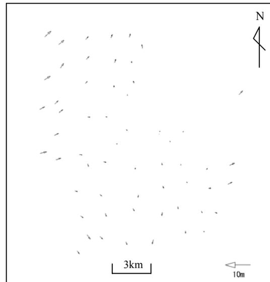
Fig.6 Horizontal component of error vectors
