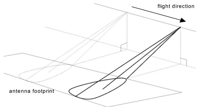
Figure 3. StripMap Geometry
