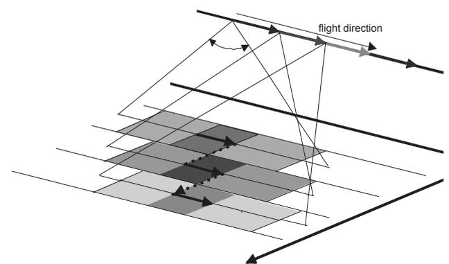
Figure 4. ScanSAR Geometry
