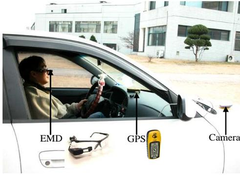
Figure 10: Hardware components of client system.
