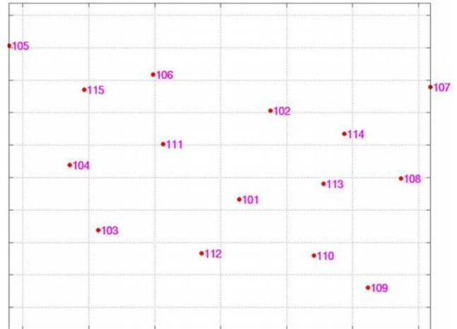
Figure 3. Distribution of 13 ground points used for the georeferencing of the stereo pair with rigorous sensor model.
