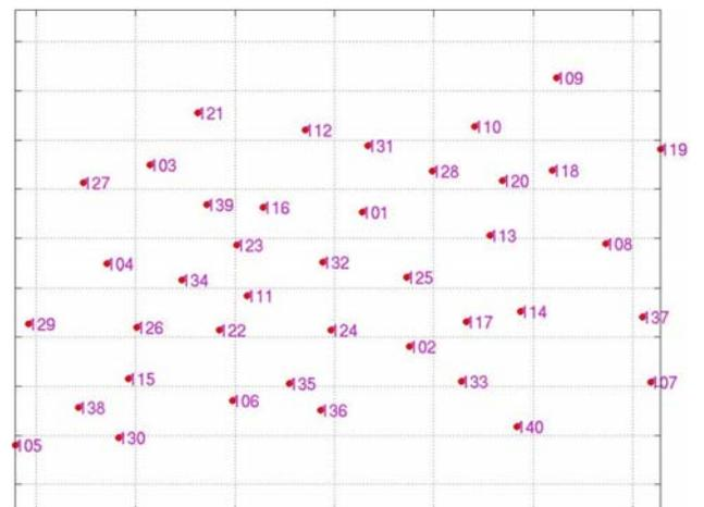
Figure 4. Distribution of 40 GCPs used to georeference one scene with RFM approach.
