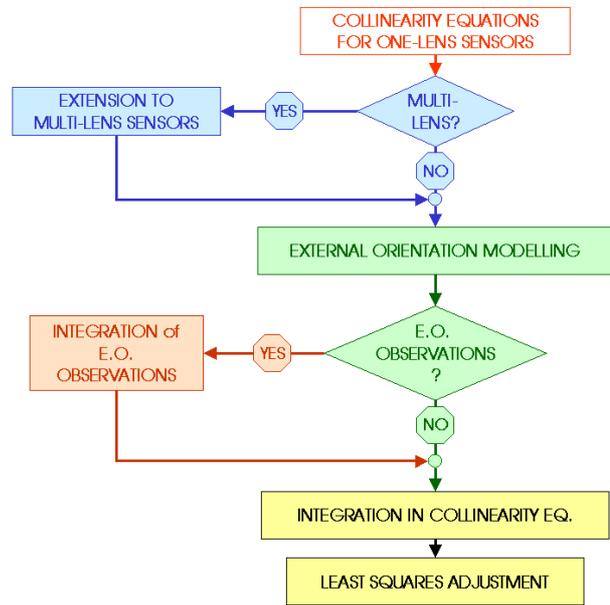
Figure 4. Overview of sensor model.
