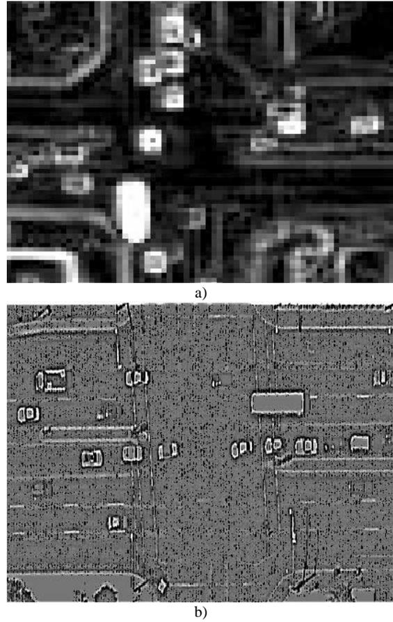
**Figure 2.** Edges extracted from 1-m satellite (a) and 15-cm airborne (b) images.
