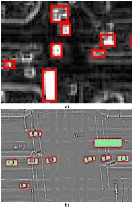
**Figure 3.** Vehicles extracted from 1-m satellite (a) and 15-cm airborne (b) images.
