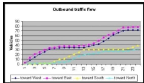
Figure 8. Flow count per traffic light in the four directions.
