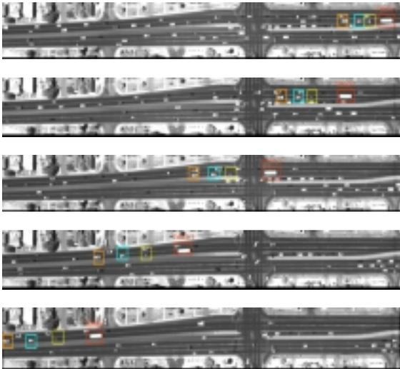
Figure 10. Tracking four moving vehicles.
