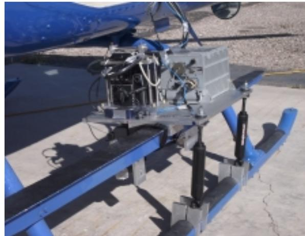
**Figure 4.** Experimental sensor configuration – 4 K by 4K digital camera with IMU and video/digital camera assembly (not visible in this image).
