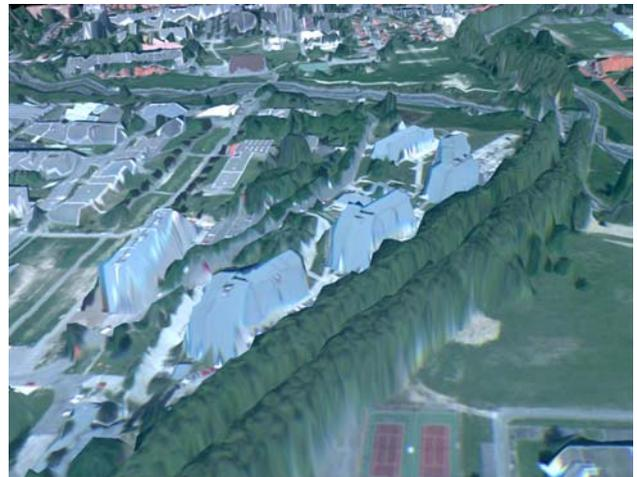
Figure 7 : Pléiades simulation draped over a 4m-DEM: vegetation looks natural, but flat roofs and roads are distorted
