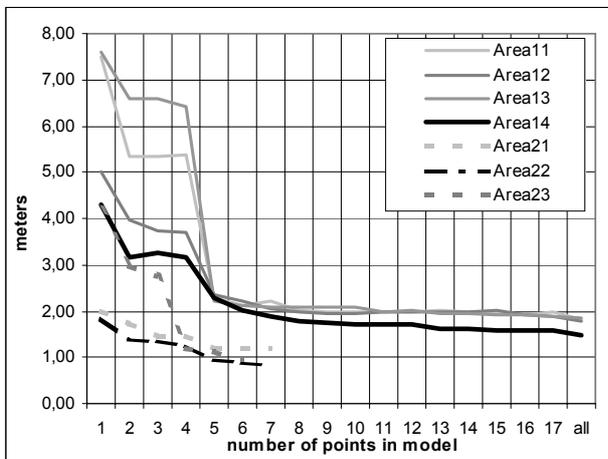
Figure 2. RMSE computed on CPs for the seven test area as function of the number of GCPs used in the model.
