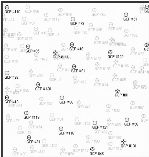
Figure 1 – Example of distribution of GCPs (in black) and CPs (in grey) for a QuickBird frame
