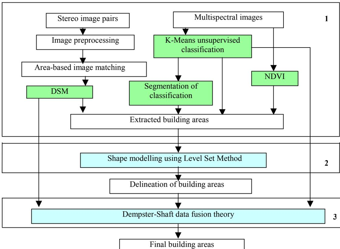
Figure 1 Architecture of the building extraction system
