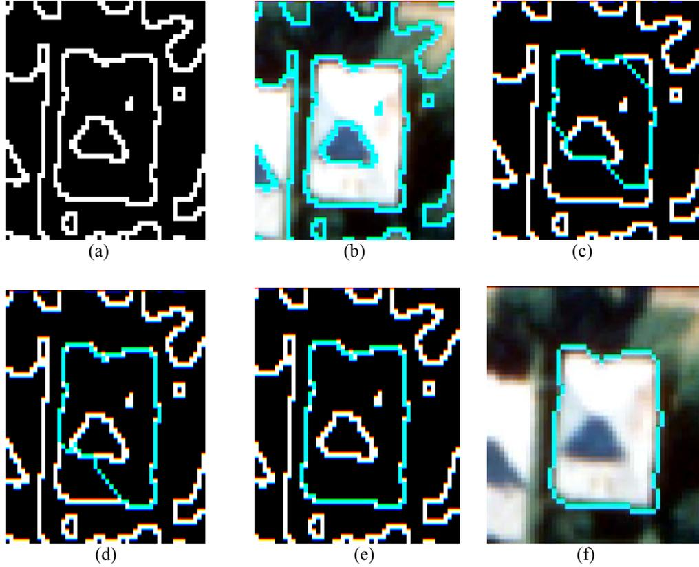
Figure 2 The example of delineation the boundary of the building area
