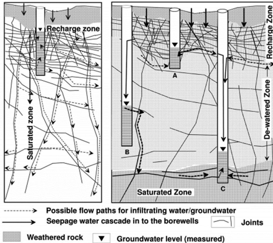
Figure 6. Conceptual model explaining the flow in fractured rock aquifer region. (a) Normal hydrogeological condition. (b) Conditions in severely exploited system. Note the flow of water from shallower borewell through an exposed joint near water level (Ballukraya and Srinivasan, 2019)
