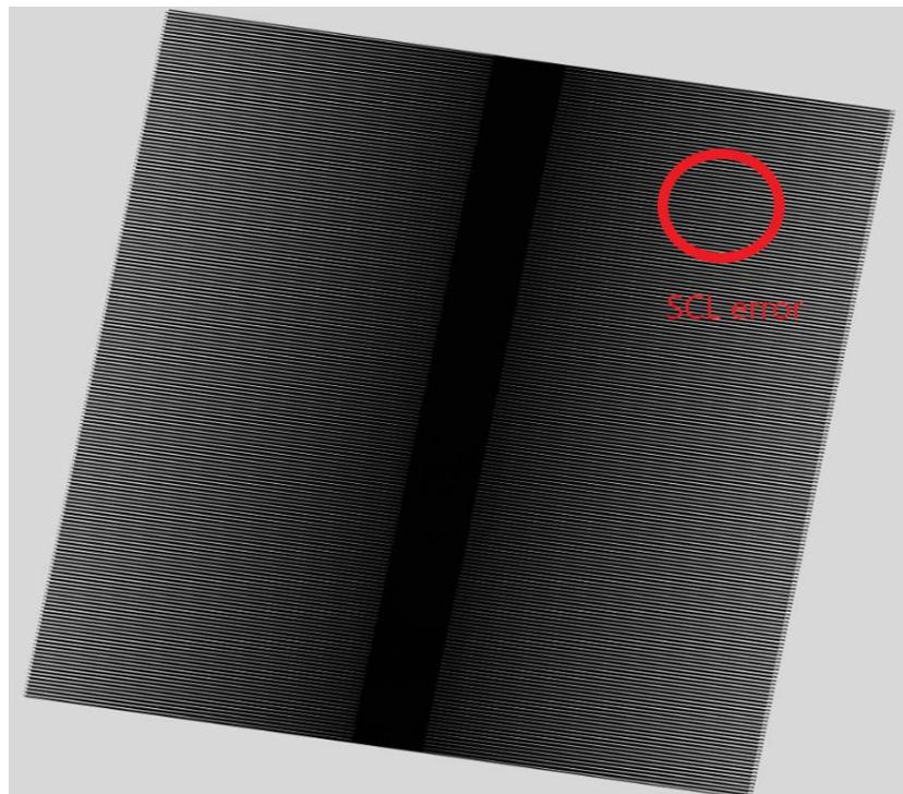
Figure 10. Pictorial representation of Scanned Line Error in Landsat-7 images.
