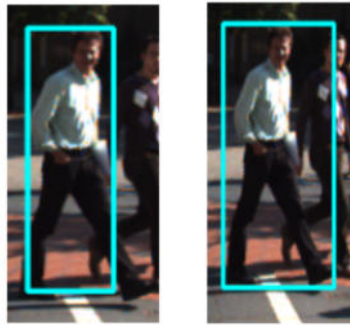
Figure 38: Left: Bounding box predicted from the previous frame using optical flow. Right: Bounding box refined after the key-frame update.
