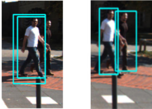
Figure 53: Left: Wrong annotations given in the ground-truth. Right: Boxes obtained by the detection algorithm (frame number: 98, sequence 16)
