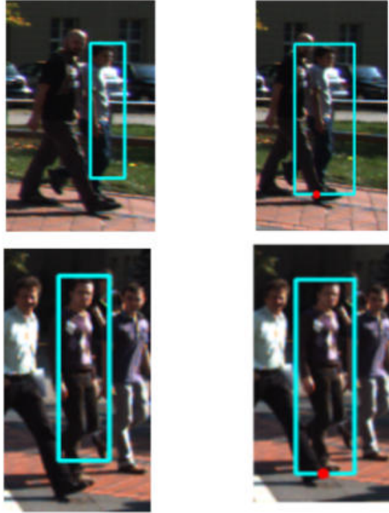
Figure 32: Left column: Bounding boxes obtained using the Mask-RCNN. Right column: Bounding boxes predicted while tracking.
