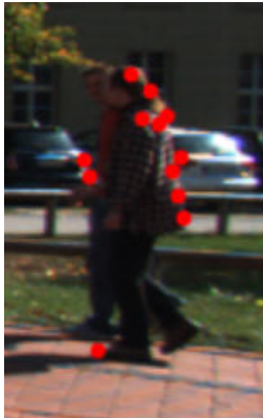
Figure 34: Points (marked in red) selected for tracking the detected pedestrian using optical flow
