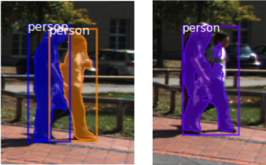
Figure 25: Left: Detections for the left frame. Right: Detection for the right frame (frame number: 28, sequence: 16)
