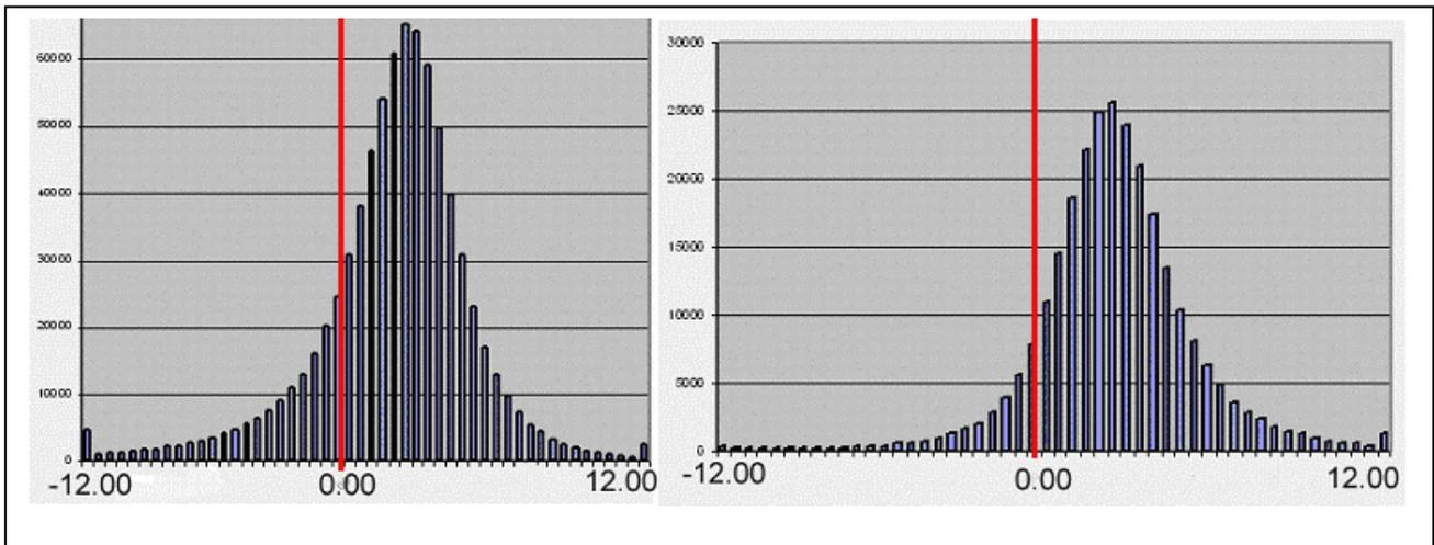
Fig. 30: on the left: distribution of frequency of DSM and on the right : DEM mountain terrain(Mausanne).
