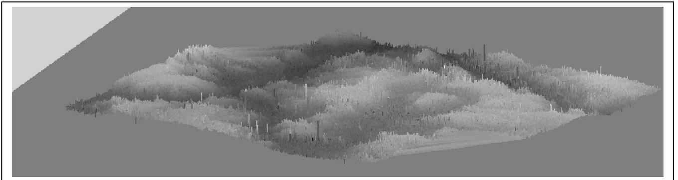
Fig. 27: DSM with  $p_y$  limit = 1.5, Warsaw scene.
