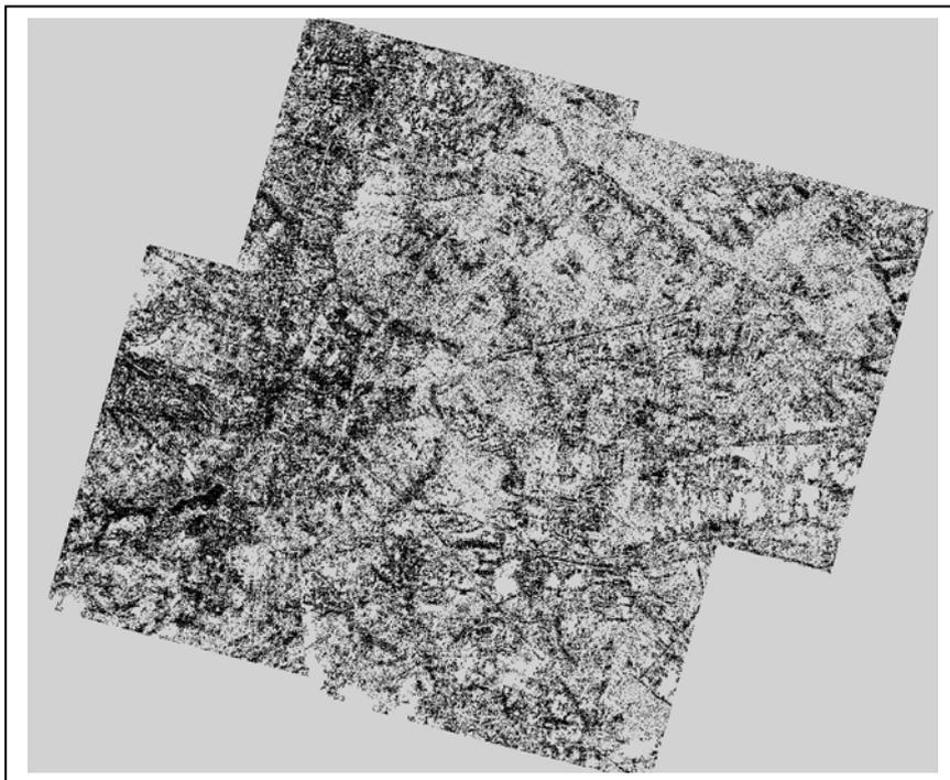
Figure 42: Binary image of Warsaw area with matching window of 25 m and interpolation distance-75 m, white = gaps in height model.
