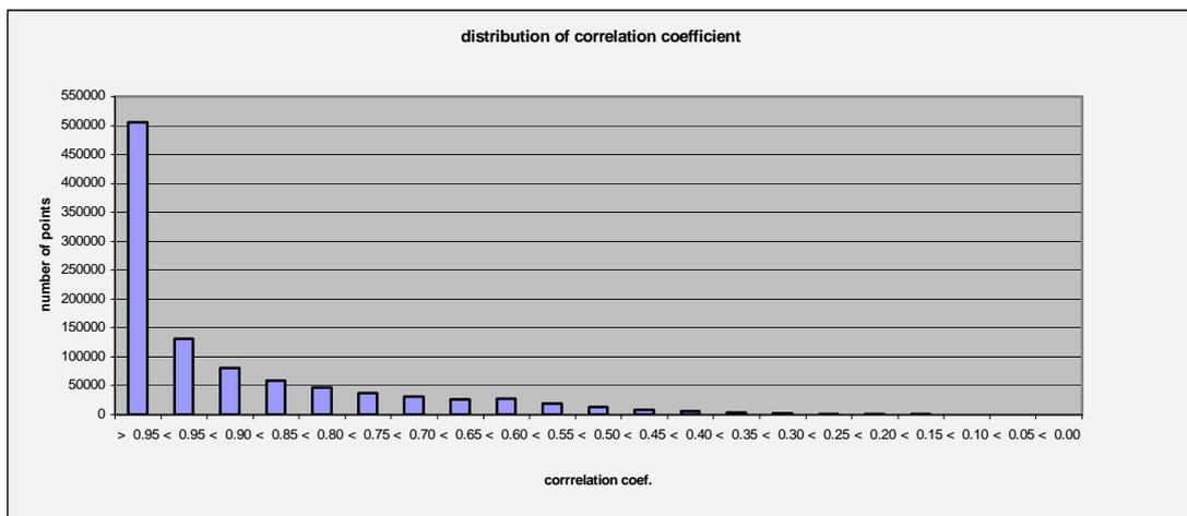
Fig.19a: Distribution of correlation coefficient (scene Warsaw) –correlation coefficient=0.6; searching window 10x10; step=3.
