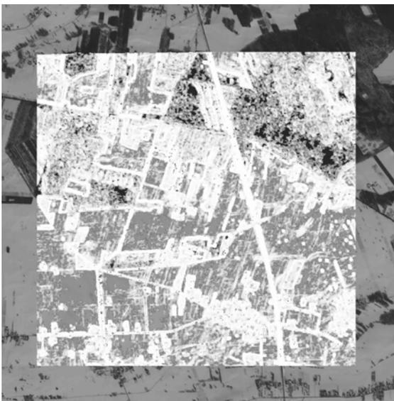
Fig.19b: Quality image: overlay of image and image points, representation of correlation coefficient as gray value(0-255) mask of matching (white color-best results gray value 1=1.0 correlation coefficient)
