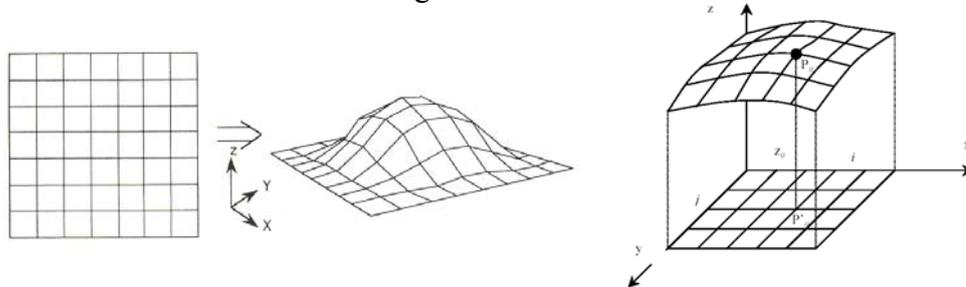
Fig. 10: GRID model. Representation of points in 2D and 3D space.
