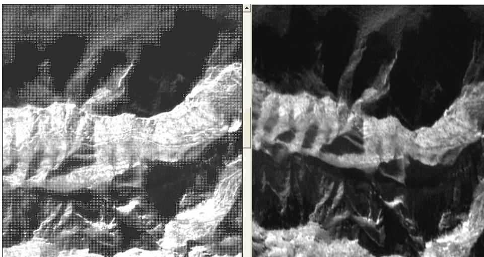
fig 20b. On the left: mask of matching. Area covered with mask represents values of correlation coefficient above threshold(0.6) and on the right original image to comparison. (Mausanne)
