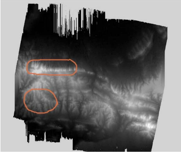
Figure 37: Problematic areas of interpolation with 30 m grid spacing and 25 m distance of interpolation.
