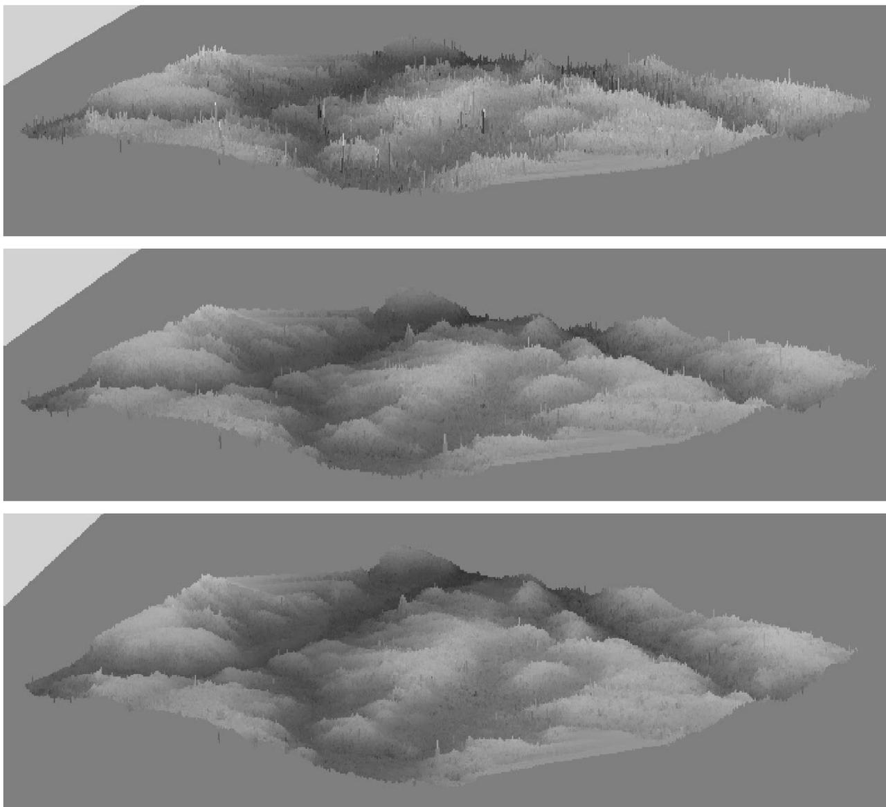
Fig. 29: From the top: DSM, DEM with the 1<sup>st</sup> iteration and with the 2<sup>nd</sup> iteration.
