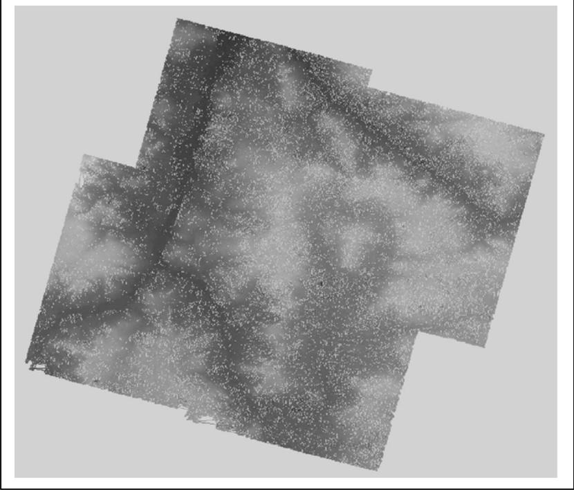
Figure 43: Image of interpolation over 25 m distance and grid size 25 m. white spaces-gaps in model.
