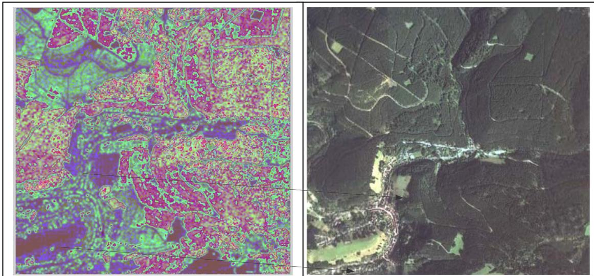
Figure 35: differential image of two files: DSM and DEM. Blue areas indicates on no differences between models (so not covered regions) and green, red, green present differences in objects heights. On the right side the same area but as satellite image.
