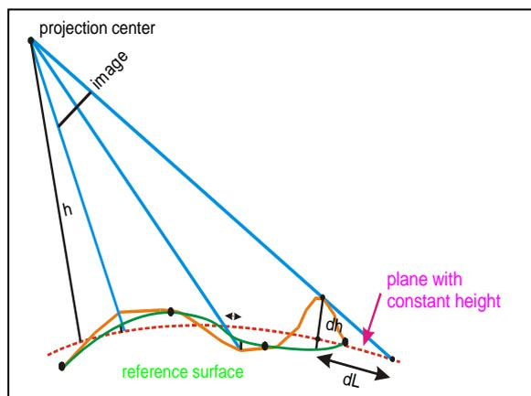
Fig. 8: Terrain relief correction.
