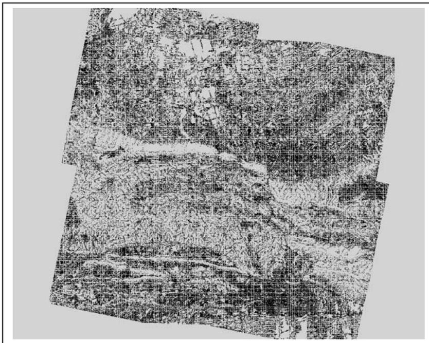
Figure 39: DEM: Mausanne area with 7.5 m grid size: binary image: white spaces: gaps in data set
