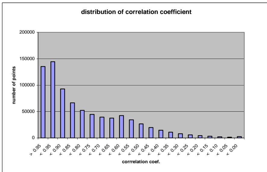
Fig. 21a: Distribution of correlation coefficient of matched points in Mausanne scene – flat area (correlation coefficient=0.6, search window=10x10).
