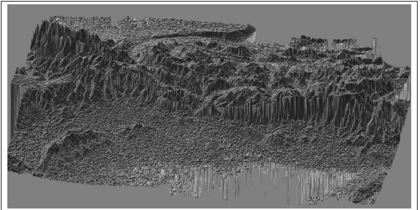
Figure 41: View on the fore-slope terrain of Mausanne data: grid size 7.5 m and interpolation distance 25m.
