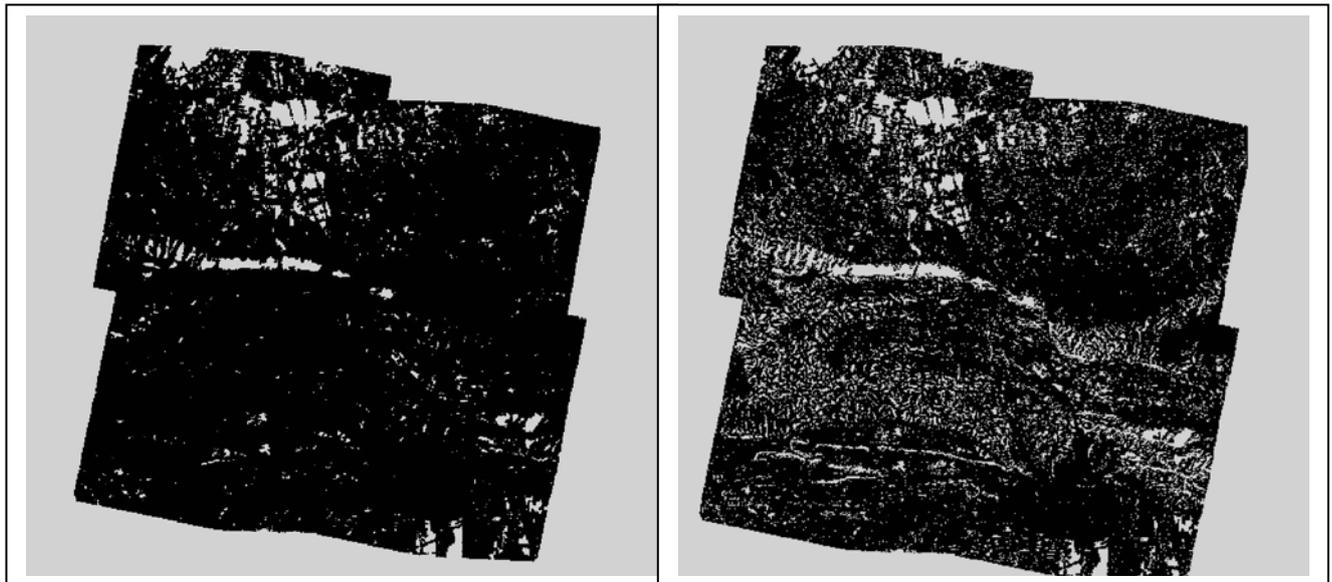
Figure 36. DSM as binary image; white spaces are gaps in model with 30 m grid size, on the right: image after filtering but without interpolation.
