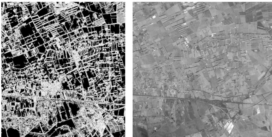
Fig. 21a: on the left: only a mask of quality image (white color best results gray value 1=1.0 correlation coefficient) on the right side original image
