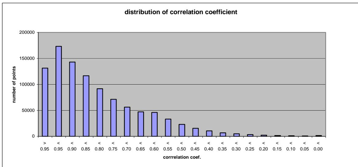
Fig 20a. Distribution of correlation coefficient of matched points in Mausanne scene mountain areas (correlation coefficient=0.6, search window 10x10, step=3).
