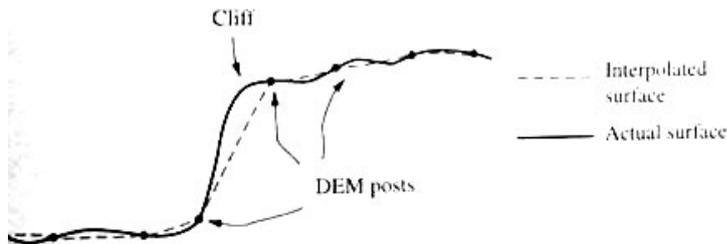
Fig. 15: example of break-line
