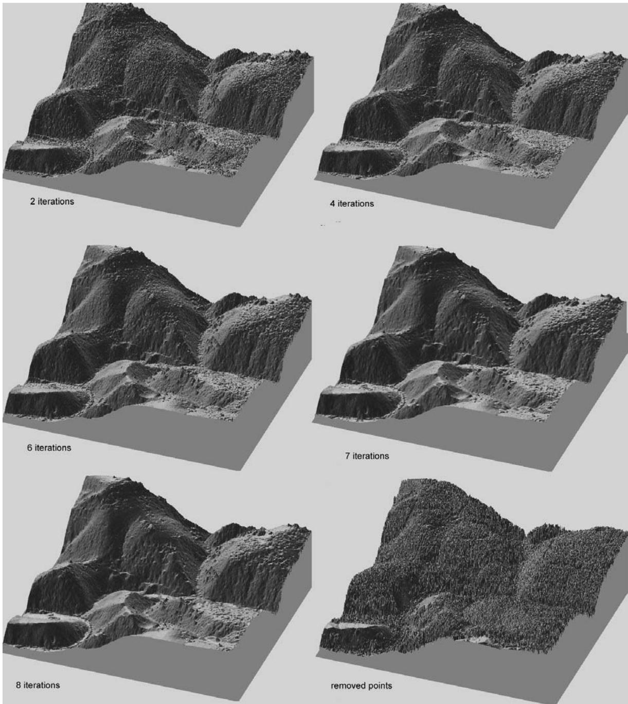
Fig 34: filtered models: from the upper left to lower right: filtering by 2/4/6/7/8 iterations, and removed object points.
