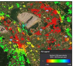
(Left) Damage at the highway A20 close to Tribsees (photo: Police Stralsund). The goal is to assess the hazard at traffic infrastructures to prevent such damages. (Right) Mean velocity deformation map around the open-pit mine Hambach in Nordrhein-Westfalen, Germany (from BodenBewegungsDienst Deutschland). Strong subsidence is threatening highways and railway tracks in the greater area around the mine.
