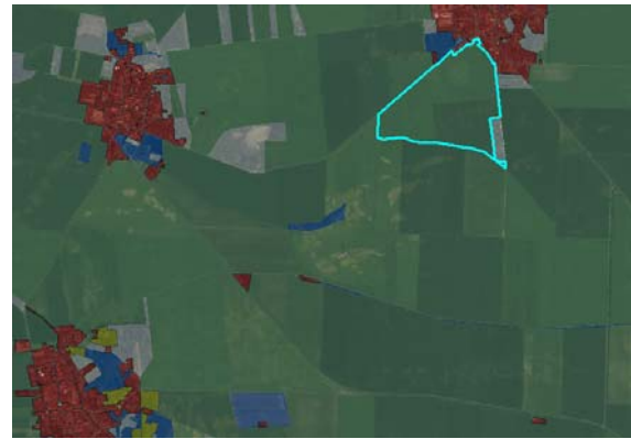
Figure 5. RGB-IKONOS image from Halberstadt with ATKIS superimposed to it (red: settlement, green: cropland, blue: grassland, yellow: forest).
