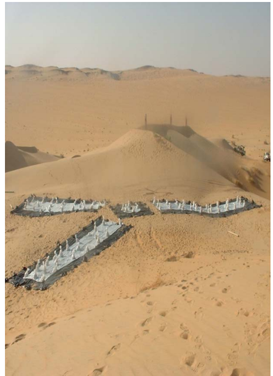
Figure 3.4: Signalized Boundary point and photo control point
