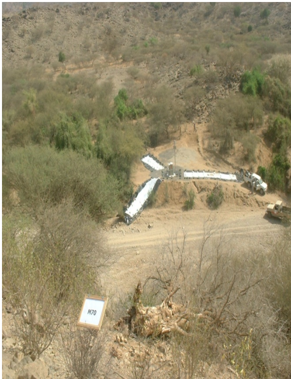
Figure 3.4: Signalized Boundary point and photo control point
