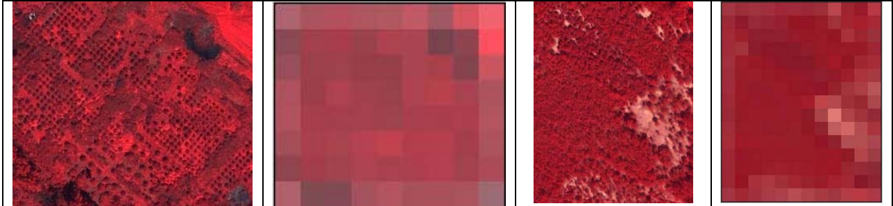
Figure 3: false color infrared images of 2 forest areas with 1m GSD and with 30m GSD
