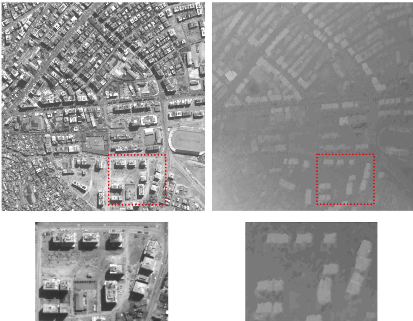
Figure 47: DSM generated by SGM algorithm; lighter gray levels correspond to higher elevations
