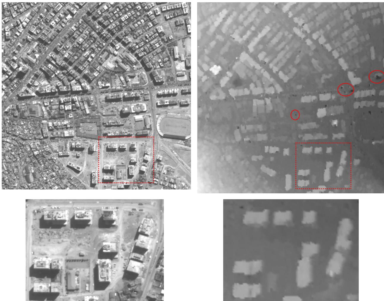
Figure 31: DSM generated by LSM algorithm; lighter gray levels correspond to higher elevations
