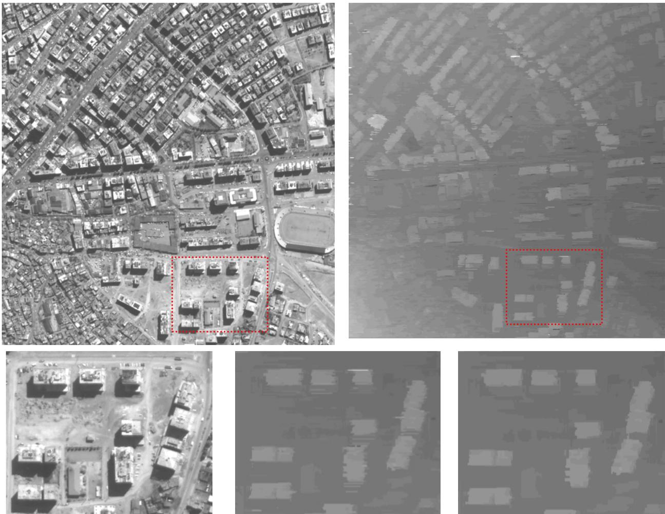
Figure 41: DSM generated by DP algorithm; lighter gray levels correspond to higher elevations Upper left: IKONOS image over Maras test area; upper right: gray value coded DSM; lower left: sub-area of IKONOS image; lower center: sub-area of gray value code DSM before vertical median filtering; Lower right: sub-area of gray value code DSM after vertical median filtering
