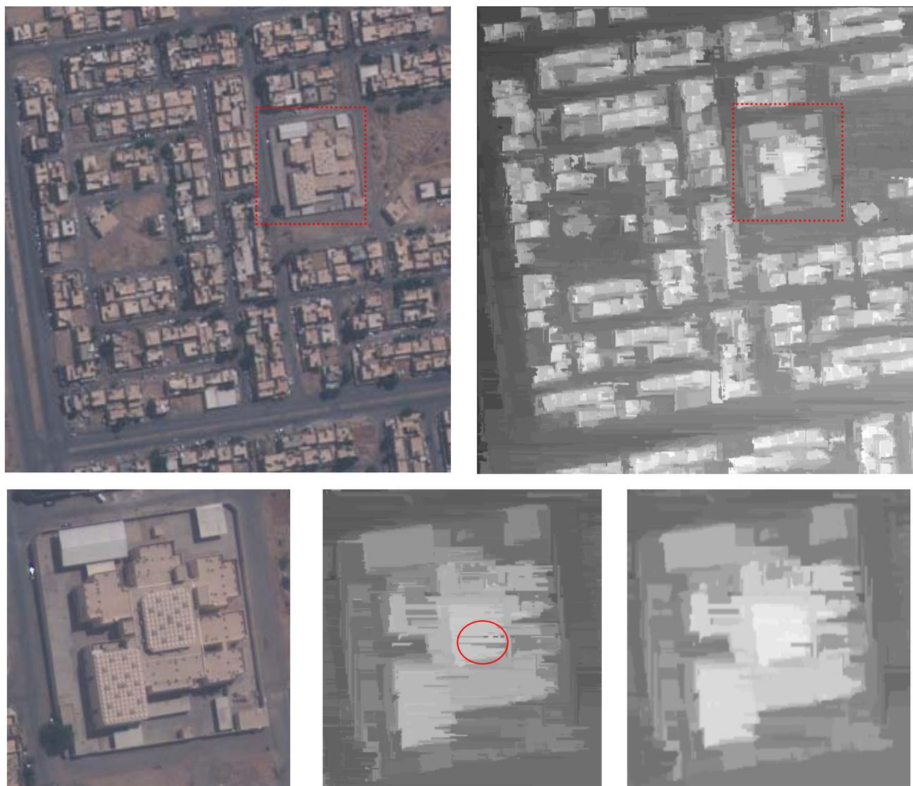
Figure 38: DSM generated by DP algorithm; lighter gray levels correspond to higher elevations Upper left: GeoEye-1 images over Riyadh test area; upper right: gray value coded DSM; lower left: sub-area of GeoEye-1 image; lower center: sub-area of gray value code DSM before vertical median filtering; Lower right: sub-area of gray value code DSM after vertical median filter
