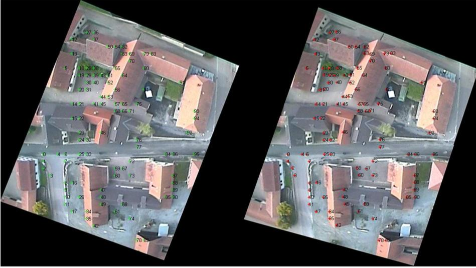
Figure 4.7: Two rectified images of the sequence Bonnland and a point set (marked in green) detected by means of (4.8) in a window of  $20 \times 20$  pixels in the left image. In the right image, correspondences obtained by the local method are marked in red.
