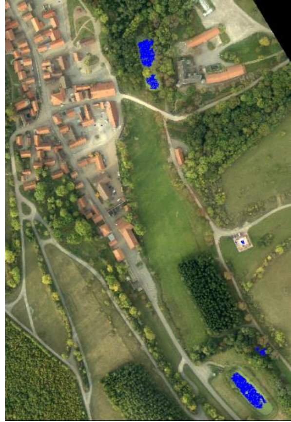
Figure 8: Orthoimage and classified water surfaces (blue) considering height variation and intensity variation
