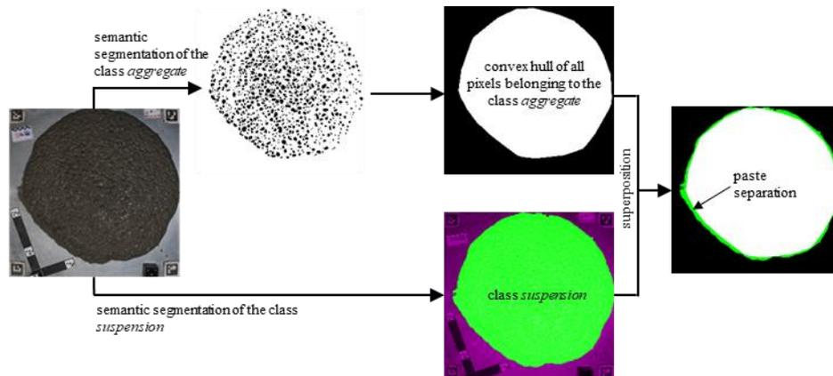
Figure 3 – Application of algorithms for semantic segmentation the classes and individual areas of the concrete spread flow (based on [44])
