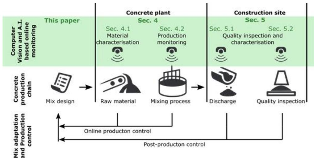
Figure 1 – Concrete production chain and AI based monitoring in the different process steps of the concrete production chain.
