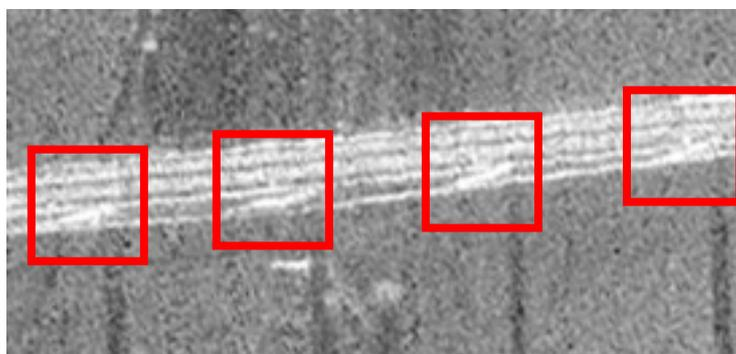
Figure 4: Bridge pillars (in red boxes) in the SAR image of the railroad bridge near Zellinger (illumination direction from top to bottom)
