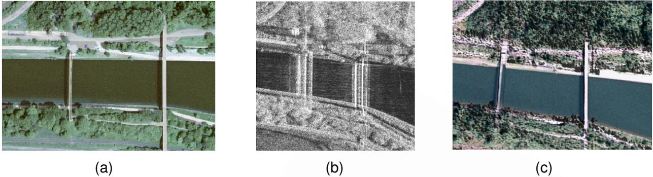
Figure 1: Test images of bridges near the city of Dorsten in southern Germany, (a) Optical aerial image, (b) InSAR magnitude image pair taken in X-Band (illumination direction from right to left), (c) 3D visualization of optical and InSAR data after fusion
