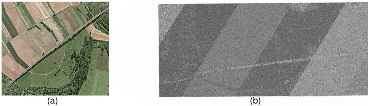
Figure 2: Test images of a railroad bridge made of concrete-steel near the city of Zellingen in southern Germany, (a) Optical image from GoogleEarth, (b) SAR image taken by the MEMPHIS sensor in X-Band (illumination direction from top to bottom)
