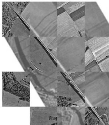
Figure 8: Checkerboard comparison of the SAR image and the optical after the registration
