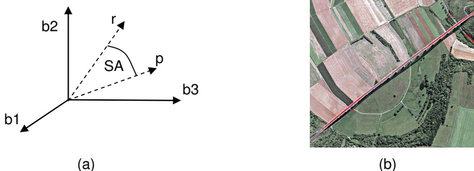
Figure 6: (a) Multi-dimensional vector space with three bands  $b1$  to  $b3$ , the vectors of the reference pixel  $r$ , the vector of the new pixel  $p$  and the spectral angle  $SA$ , (b) Optical aerial image of the railroad bridge overlaid with the extracted lines (red)
