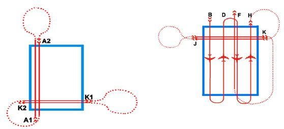
Figure 1: Calibration flight, image scale 1:5000
