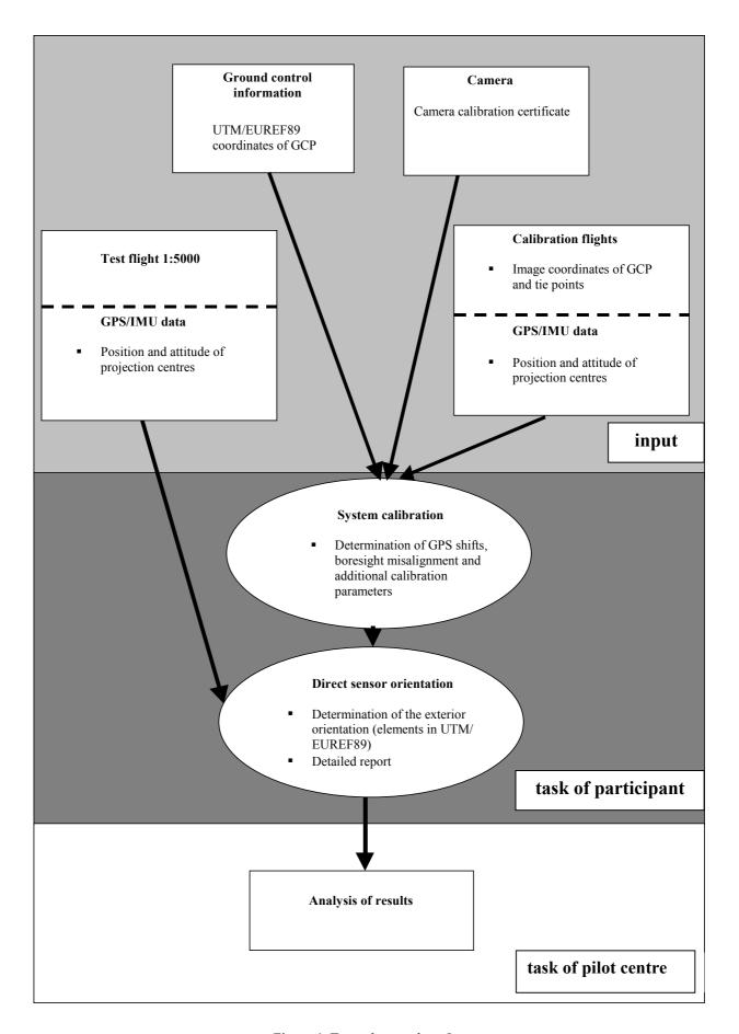
Figure 4: Test scheme, phase I
