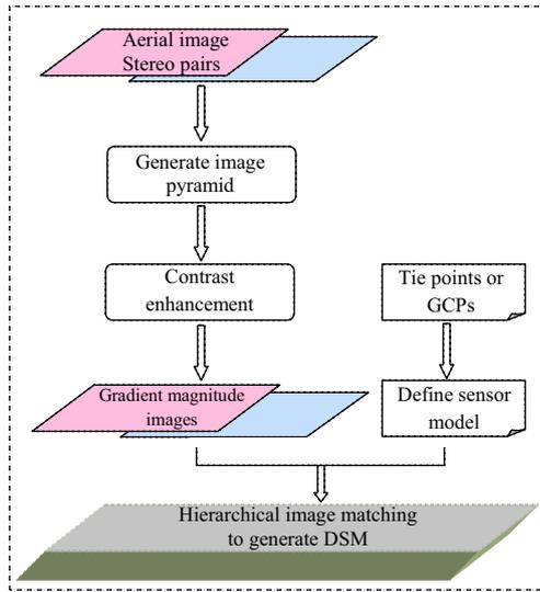
Figure 3. Working process of DSM generation.
