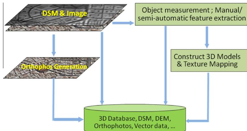
Figure 4. Workflow of the 3D building generation.
