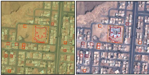
Figure 11. Updated map overlaid with aerial orthophoto of 2007 (left) and GeoEye-1 orthophoto from 2010 used for mapping (right)
