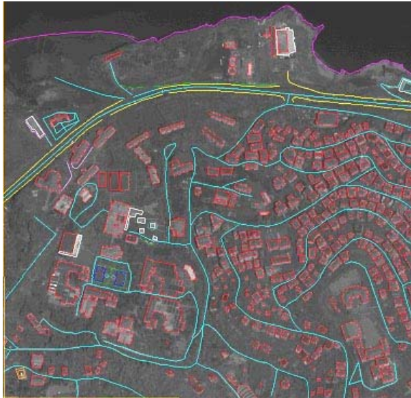
Mapping results based on OrbView-3 panchromatic image buildings which could be identified but not vectorized are shown as cross
