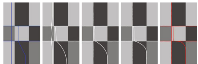
Fig. 10 Optimization of network snakes exploiting a wrong topology with one missing contour part: initialization (blue), optimization steps (white) and result (red)
