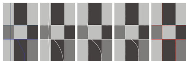
Fig. 11 Optimization of network snakes exploiting a wrong topology with two adjacent missing contour parts: initialization (blue), optimization steps (white) and result (red)
