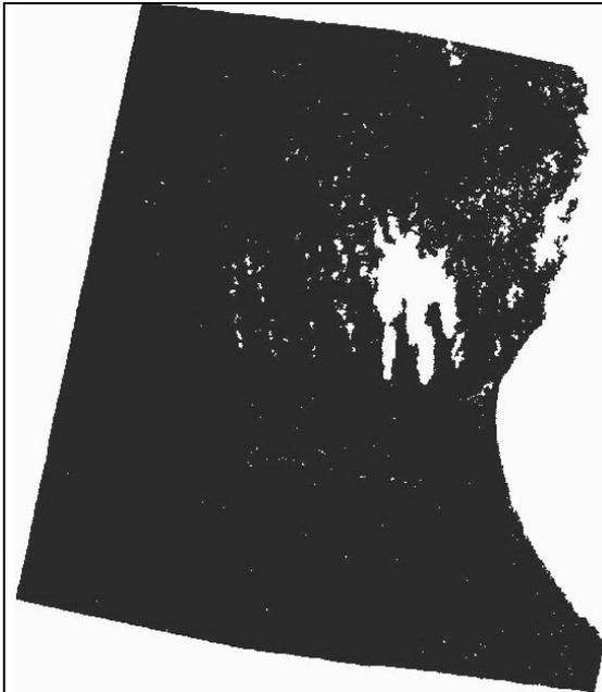
Figure 1: object points determined by matching of Cartosat-1 stereo pair Istiranca (black), not covered area mainly influenced by clouds
