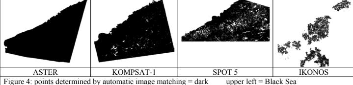
With the exception of ASTER all height models do have some gaps. Of course no points are available from the sea - a matching of the sea surface with moving waves and different sun reflection is not possible. The matching of TK350 photos was influenced by the film grain and several scratches on the film requiring a scratch removal filtering. But also after filtering the results especially in the forest areas could not be accepted, it was influenced by very low contrast.
