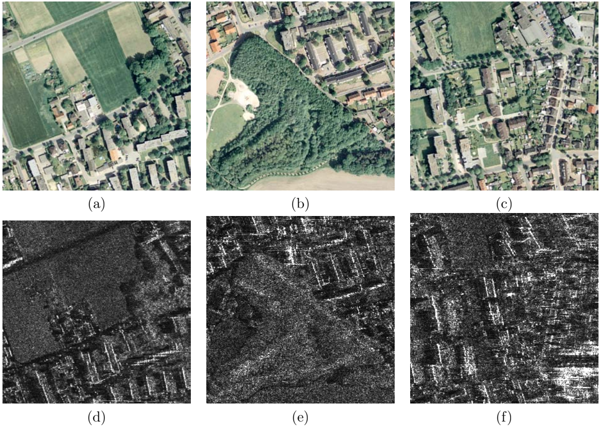
Figure 4.3.: (a)-(c) Subscenes of the optical orthophoto (Fig. 4.1) and (d)-(f) corresponding subscenes of one SAR magnitude image (Fig. 4.2) of the interferometric pair.
