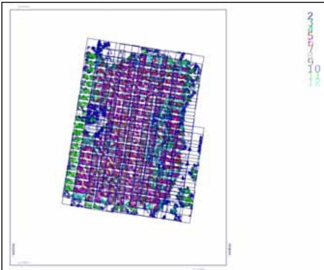
Fig. 8: block configuration with all used images, object points colored by number of images/point – color coding see upper right
