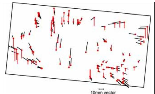
Fig. 17: Deformation of model 206/207 caused by systematic image errors, red vectors = Z-discrepancies
