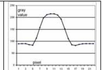
Fig. 6: gray value cross-section through traffic separator
