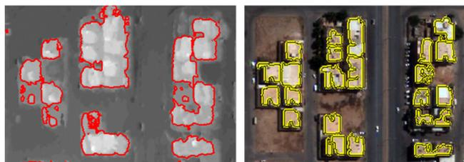
Fig. 1. Extraction of building footprint using (left): height threshold on nDSM derived from image matching, (right): segmentation of building rooftops over a GeoEye image using the level set approach
