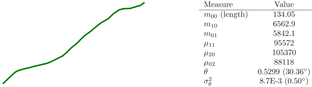
Figure A.4.: Examples of line moments: zeroth and first order: normal moments; second order: translation invariants and \theta derived from them. The variance of \theta is based on an assumed variance of the object coordinates \sigma_{x,y} = 0.8m .
