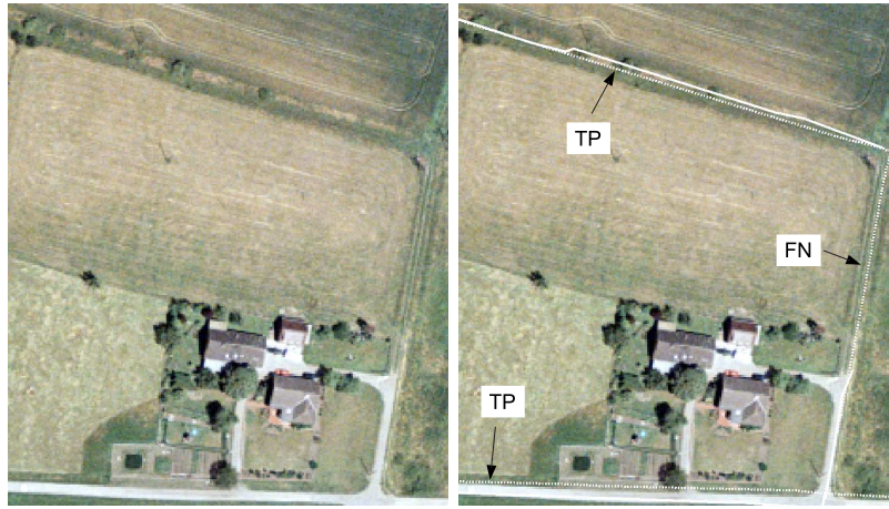
Figure 4.12.: Example for True Positive and False Negative decision, obtained with roads resulting from parameter set 1. The dashed lines show three road objects; two of them are correct and accepted (True Positive, TP), one is correct, but rejected (False Negative, FN).
