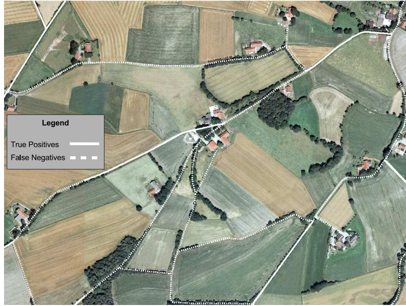
Figure 4.15.: Example for False Negative decisions resulting from occlusions caused by rows of trees
