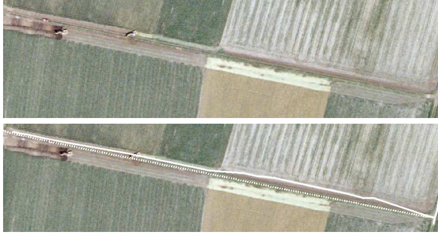
Figure 4.9.: Example for False Positive decision. Upper image: orthoimage detail showing a road under construction; lower image: superimposed extracted road (continuous line) and ATKIS road object (dashed line).
