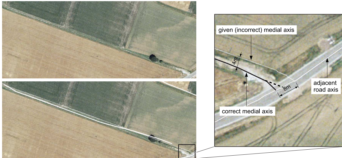
Figure 4.10.: Example for False Positive decision. Left, upper image: orthoimage detail showing a path leading to a field; left, lower image: superimposed extracted road (continuous line) and ATKIS road object (dashed line). The magnification (right) shows the correct road axis. The ATKIS road object is not correctly connected to the adjacent road at the right side.
